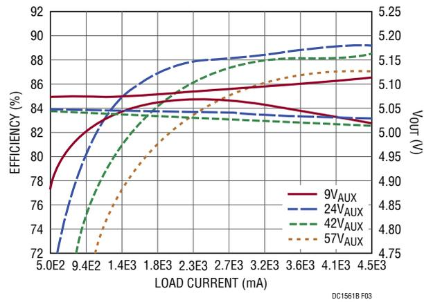
Figure 3. Efficiency and Regulation (Including OR'ing Diode, D12)
