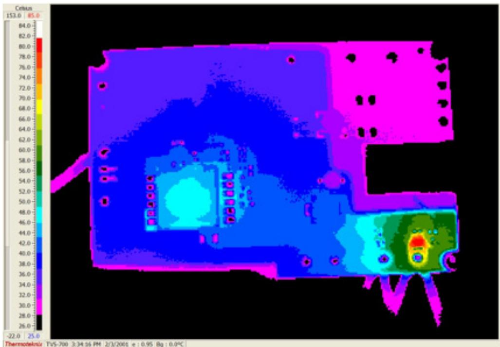
Figure 7. Temperature Data (9V<sub>AUX</sub>, 4.5A, Bottom)
