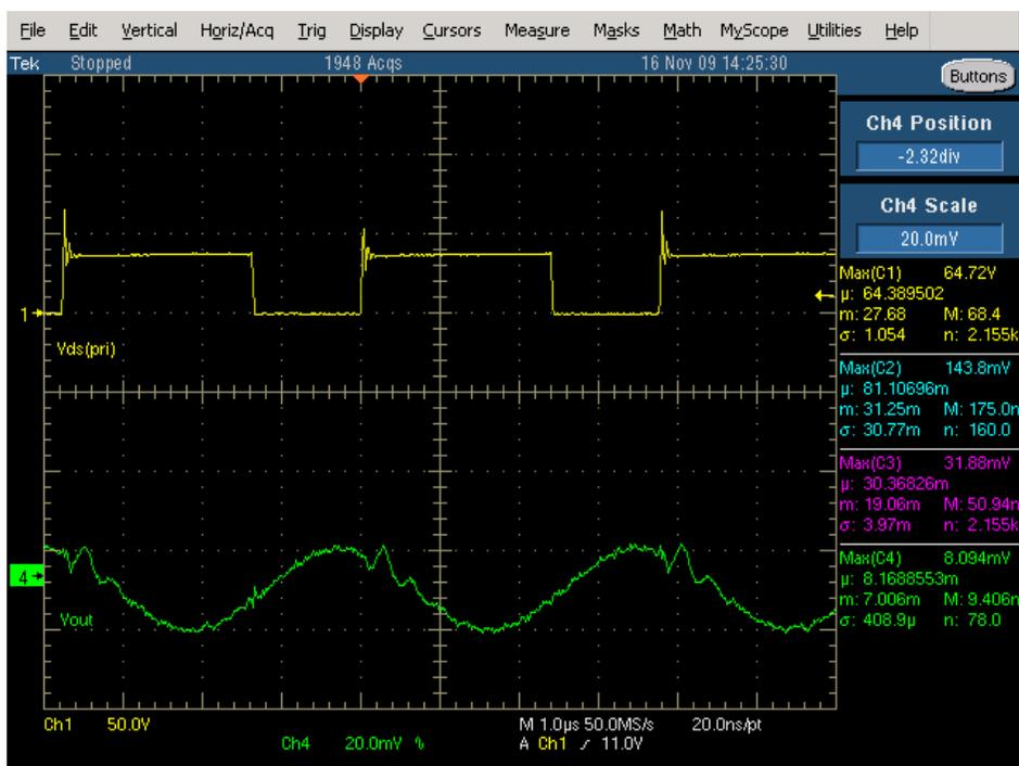
Figure 4. Output Ripple (24V<sub>AUX</sub>, 4.5A)
