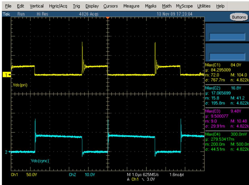
Figure 10. Stresses (9V<sub>AUX</sub>, 4.5A)
