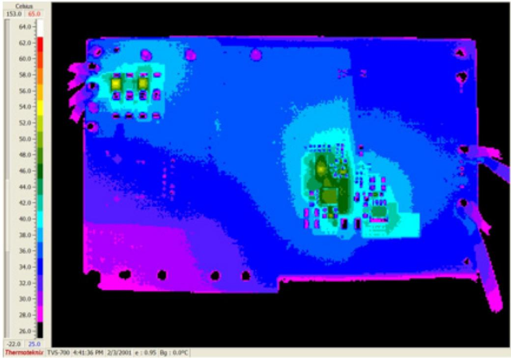
Figure 8. Temperature Data (37V<sub>PORT</sub>, 4.5A, Top)
