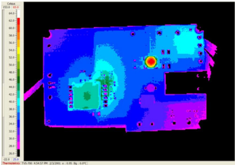
Figure 9. Temperature Data (37V<sub>PORT</sub>, 4.5A, Bottom)
