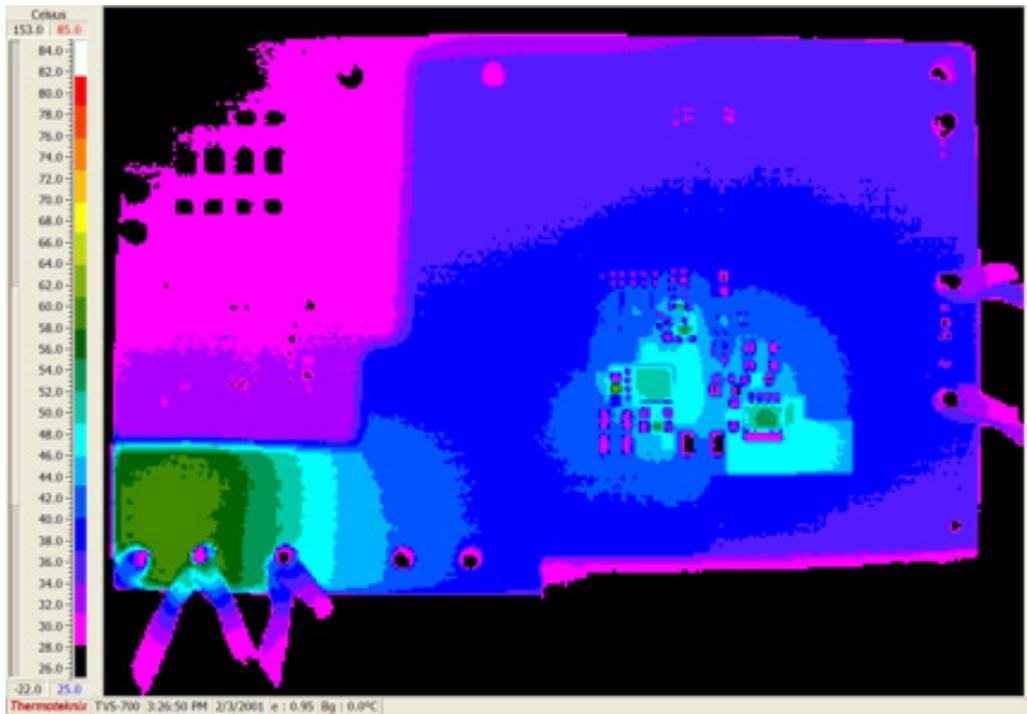
Figure 6. Temperature Data (9V<sub>AUX</sub>, 4.5A, Top)
