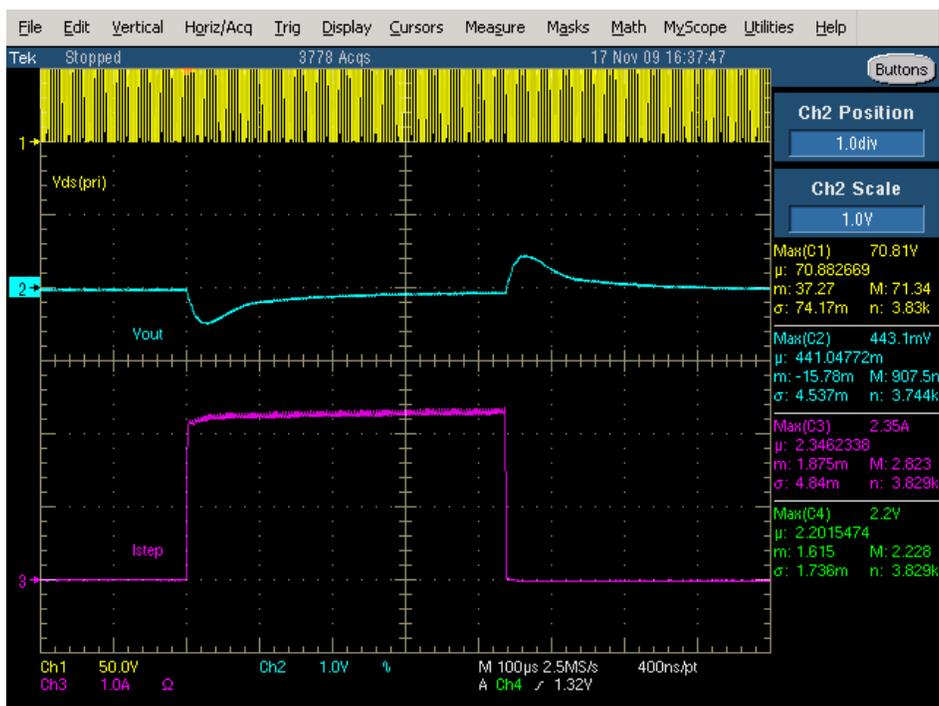
Figure 5. Load Transient Response (57V<sub>PORT</sub>, 2.25A to 4.5A to 2.25A)
