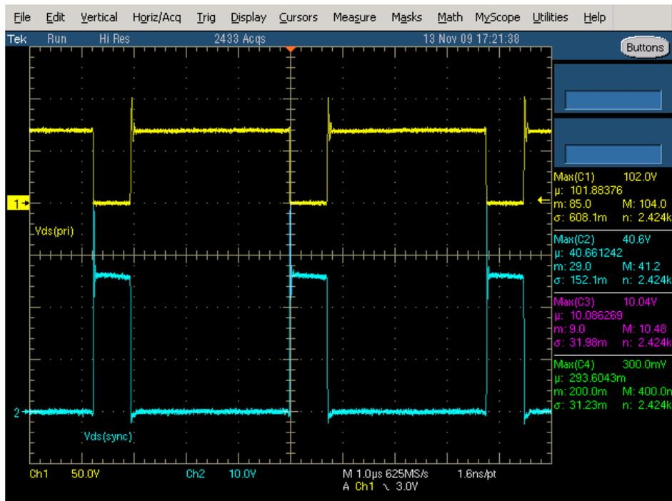
Figure 11. Stresses (57V<sub>AUX</sub>, 4.5A)
